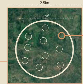
Within each tile, random centroid locations are generated for clusters. **Clusters [1km²]** are the basic sampling units and are made up of 10 **plots [1000m²]**. Using each cluster centrepoint, the sampling plots are randomized.
