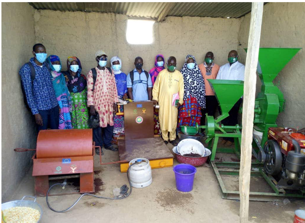
Figure 5. Shea butter production unit in the rural Municipality of M'Pessoba, Cercle de Koutiala, Mali. The kit is composed of a mill crusher–grinder, a gas roaster and a 500 Kg scale. Photo: Aboubacar Diarra/OXFAM/Mali.
