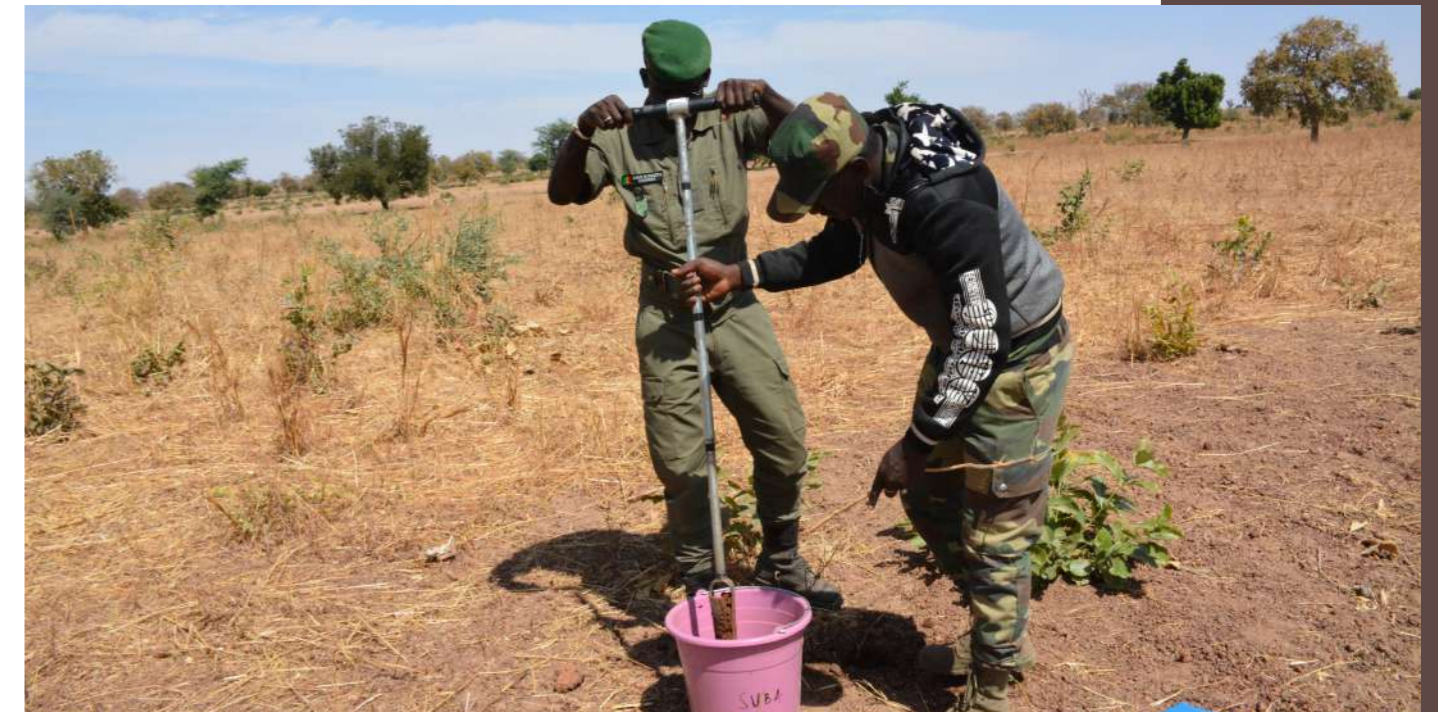
Photo: Gilberte Koffi, World Agroforestry / Officials from the Forest Department in Senegal taking soil samples for analysis of soil organic carbon and other land degradation indicators.
