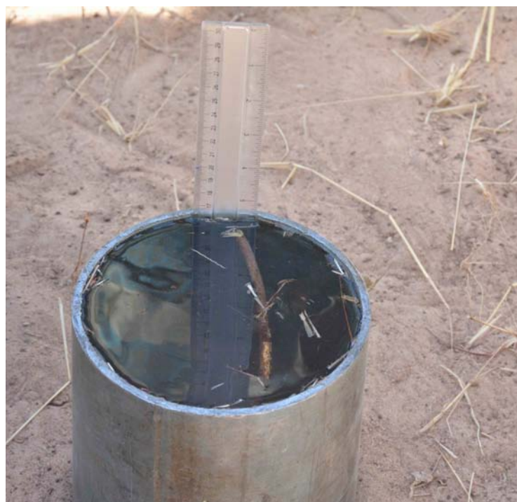
Figure 19: Photo of the single ring infiltrometer used to measure infiltration in the field. Photo: G. Koffi/ICRAF.
