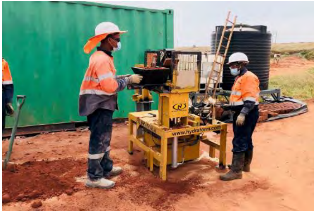
Interlocking brick making
